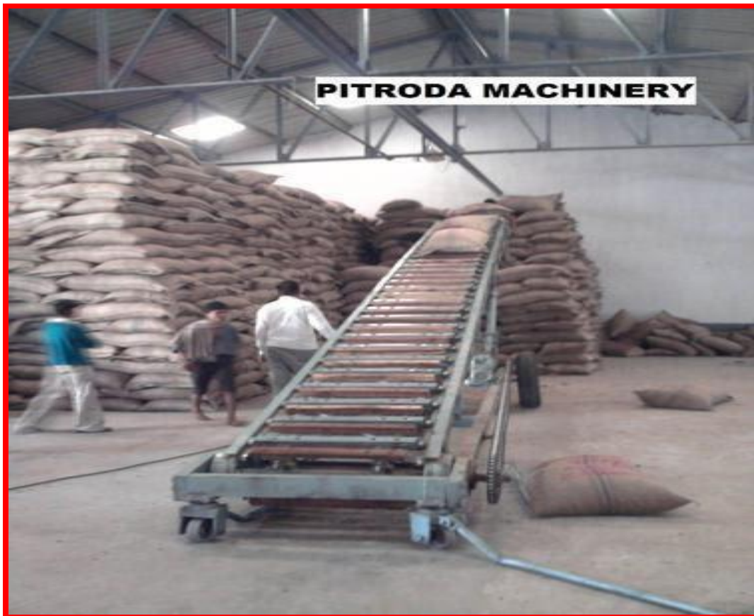
Figure 12: Loading and Unloading conveyor
